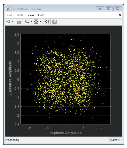
Demodulate the noisy symbols to obtain soft bits. Convolutionally decode the soft bits. Display the number of erroneous bits.
