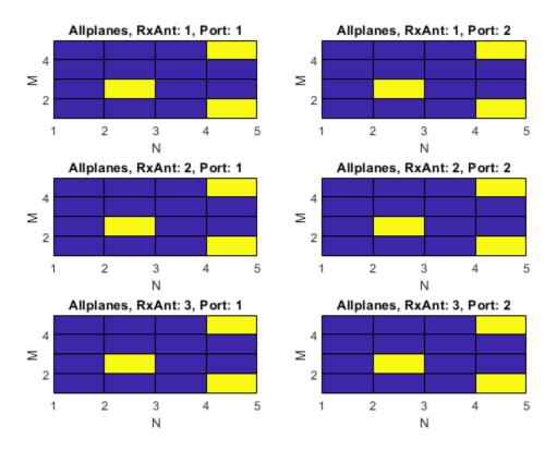
Create a 4D channel estimate grid to extract resource elements. Extract resource elements from the channel estimate grid using 'direct' extraction mode. Show the locations of these extracted resource elements. Addressed resource element locations contain 1.
