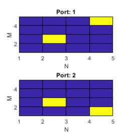
Create a 3D received grid to extract resource elements. Extract resource elements from the received grid. Show the locations of these extracted resource elements. Addressed resource element locations contain 1.
